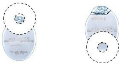
Figure 2. Correct positioning of a ring magnet to deactivate therapies of a St Jude Medical ICD
