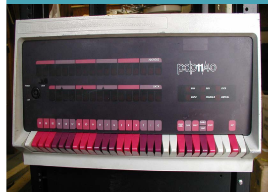
The PDP-11 computer that initially held the National Pacemaker Registry had 16k RAM and no keyboard.
